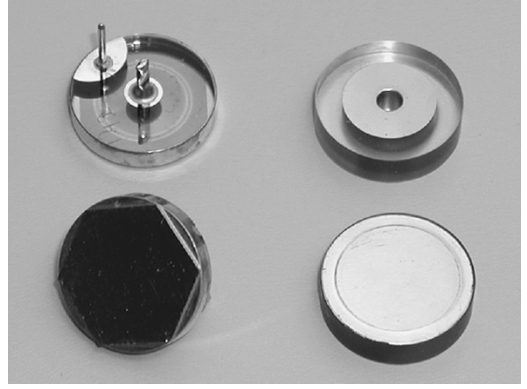
Fig. 12. Pressure sensors with silicon diaphragms (right) and polycarbonate membranes (left). The sensors are 19 mm in diameter.
